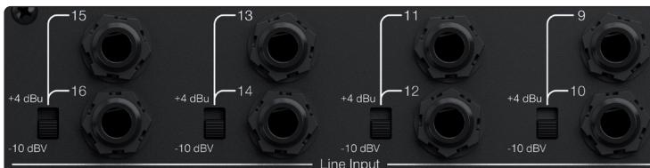
**Line Input Level (Ch 9 - 16)** - Use the two-way line input level switch to set the nominal level of adjacent Line Inputs to -10 dBV or +4 dBu.
