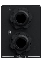
**Main Outputs (Ch 1 - 2, Left and Right)** - Use Main L and R to connect to your primary set of studio monitors.
