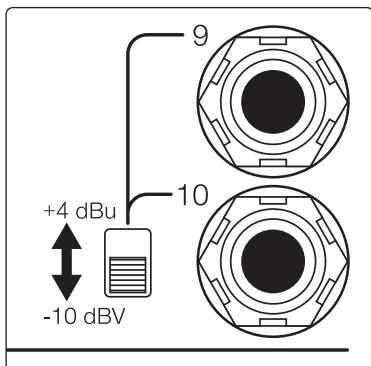
The rear-panel line level inputs (Ch 9 - 16) can be set in pairs for either +4 dBu or -10 dBV operation.
