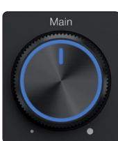
**Main Volume Knob** - The Volume Knob controls the volume level of the Main L/R outputs (outputs 1 and 2).
