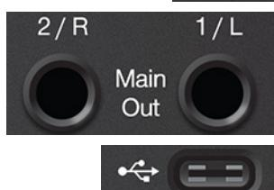
**Main Outs.** These are the Main outputs for the AudioBox Go. The output level of the Main outputs is controlled by the Main level control on the front of the unit. Playback streams 1 and 2 are routed to these outputs.
