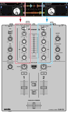
The signals played on the Serato DJ software's decks [**DECK1**] to [**DECK2**] are input to this unit's respective channels.
