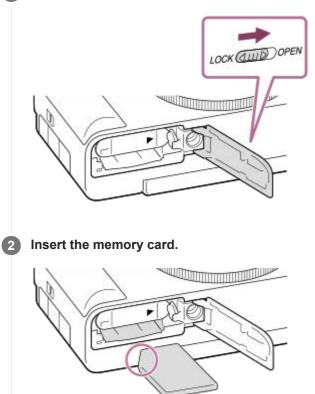
With the notched corner facing in the direction illustrated, insert the memory card until it clicks into place. Insert the memory card correctly. Not doing so may cause a malfunction.
