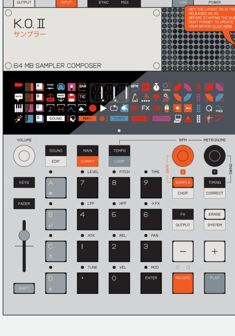
EP-133 K.O.II IS A 64 MB SAMPLER AND COMPOSER. JUST LIKE ITS POCKET-SIZED PREDECESSOR PO-33 K.O.I, THIS SAMPLER IS A MIGHTY CONTENDER ON THE STAGE, IN THE STUDIO AND IN THE RING. SAMPLE DIRECTLY FROM YOUR FAVORITE SOURCE USING THE BUILT IN MIC OR 3.5 MM INPUT JACK.
