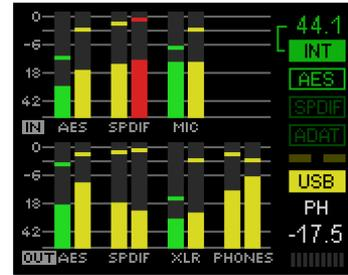
Turning the knob displays the volume screen of the currently selected output. Pressing the knob toggles the display between *Main Out* (Analog Out 1/2, XLR) and *Phones* (TRS front). At the bottom right, the current selection and dB value of the Volume setting is shown, so it is visible even when the Volume screen is not active.
