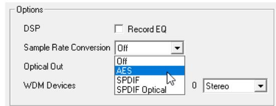
The SRC offers a maximum conversion rate of 1:7 or 7:1, respectively. Thus, 192 kHz can be converted to any sample rate down to 32 kHz, and vice versa.
