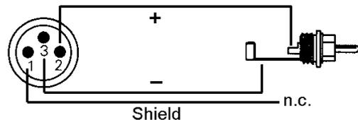
Using the cable adapter XLR/RCA described above, devices with coaxial SPDIF interface can be connected to the AES output of the Digiface AES as well. Note that most consumer equipment with phono (SPDIF) inputs will only accept signals having a Channel Status *Consumer*. In such cases the above adapter cable will not work.
