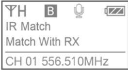
**IR Match:** Set to match with the receiver. The screen will display "Matching" when in process. After successful matching, it will read "Match success."
