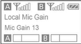
**MIC GAIN:** Adjust the external microphone's gain level (0-15). Default is "13".
