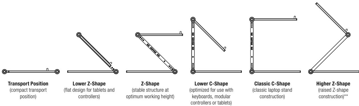
\*\* To use the Higher-Z-Shape design, you must screw the locking pins -4- into thread B -5b-.
