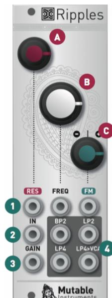
**A. Resonance level.** Self-oscillation occurs at about 80% of the course of this potentiometer.
